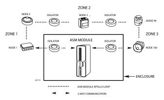
Figure 4—Class X Pathway (multi-zone with isolators)
