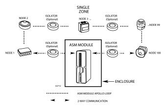
Figure 2—Class A Pathway (isolators are optional)
