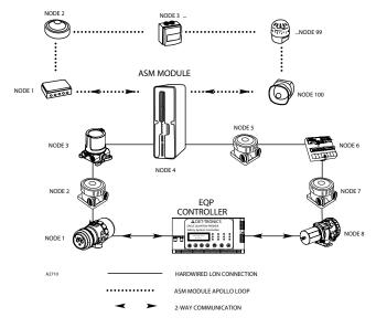
Figure 1—EQP LON with ASM Module Communication
