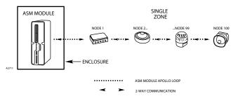
Figure 3—Class B Pathway (without isolators)
