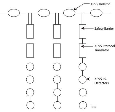
Figure 9—XP95 Wiring Schematic
