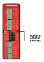
Figure 8—Location of Network Address Switches
