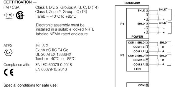
The EQ3760ASM shall be used in an area of no more than pollution degree 2 per IEC 60664-1, and in an enclosure with a tool removal cover that complies with all relevant requirements of EN 60079-15, rated at least IP54, and be connected to supply circuits where the rated voltage cannot be exceeded by 40% caused by transient disturbances.
